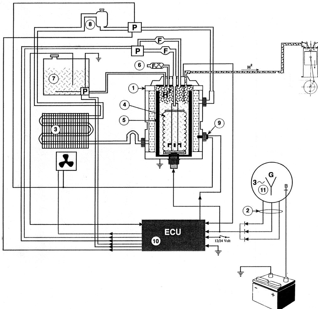
Fig. 1. General structure of the system (1. Electrolysis cell; 2. Secondary circuitry; 3. Radiator; 4. Anode electrode; 5. Cathode electrode; 6. Air filter; 7. Water tank; 8. Cooling water tank; 9. Water temperature sensor; 10. Electronic control unit of the system; 11. Alternator. P — water pump; F — water filter).
