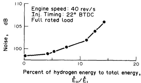
Fig. 4. Engine speed 40 rev/s, injection timing 22°BTDC, full rated load.
