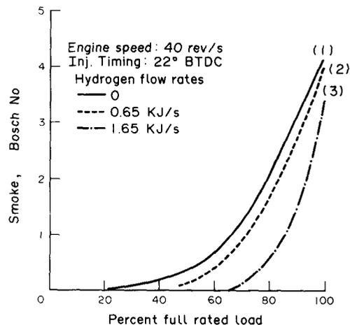
Fig. 9. Engine speed 40 rev/s, injection timing 22°BTDC. Hydrogen energy flow rates (1) 0, (2) 0.65 KJ/s, (3) 1.65 KJ/s.
