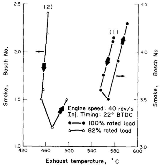
Fig. 8. Engine speed 40 rev/s, injection timing 22°BTDC. (1) 100% rated load, (2) 82% rated load.
