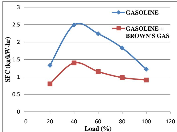
Figure 6: Comparison of Specific Fuel Consumption
