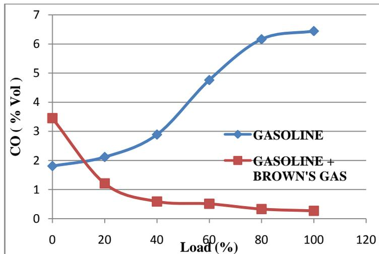
Figure 8: Comparison of Carbon Monoxide
