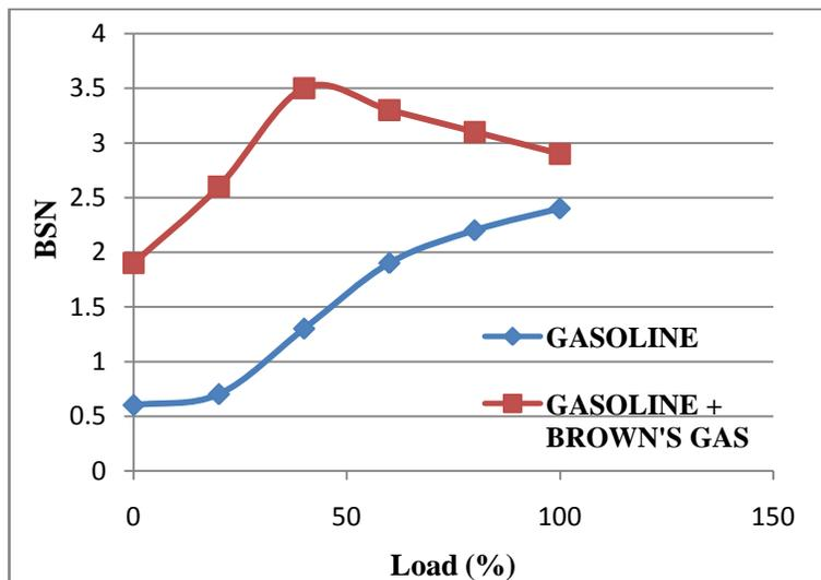
Figure 10: Comparison of Smoke Emission
