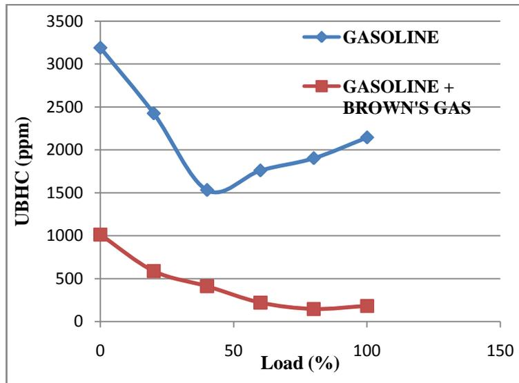
Figure 7: Comparison of Unburnt Hydrocarbon
