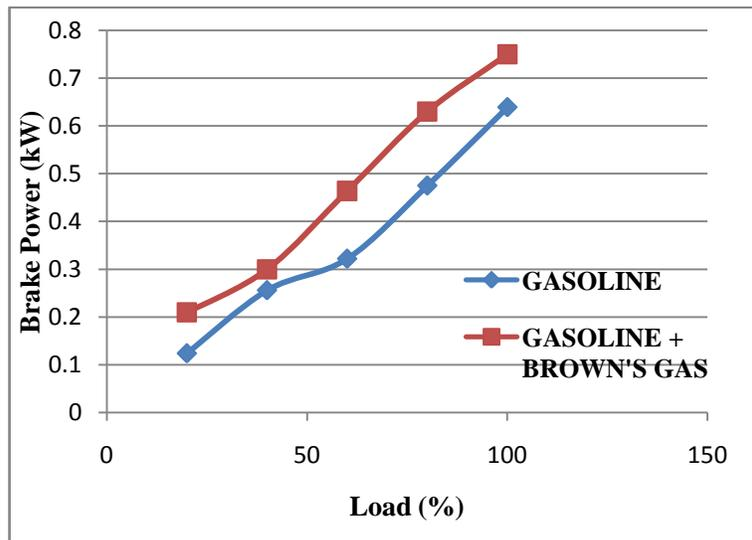
Figure 3: Comparison of Brake Power
