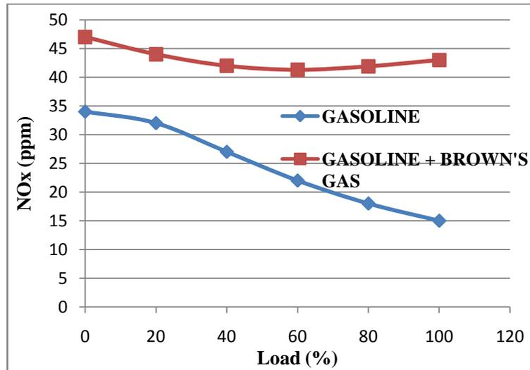
Figure 9: Comparison of Oxides of Nitrogen
