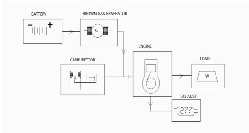
Figure 2: Experimental set up of the Test Engine
