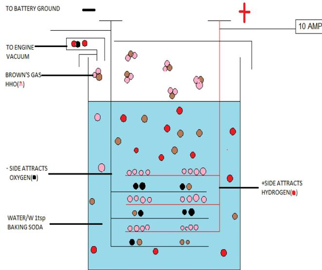
Figure 1: Schematic of Brown’s Gas Electrolyzer
