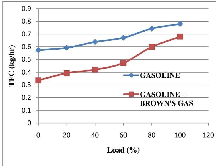
Figure 5: Comparison of Total Fuel Consumption
